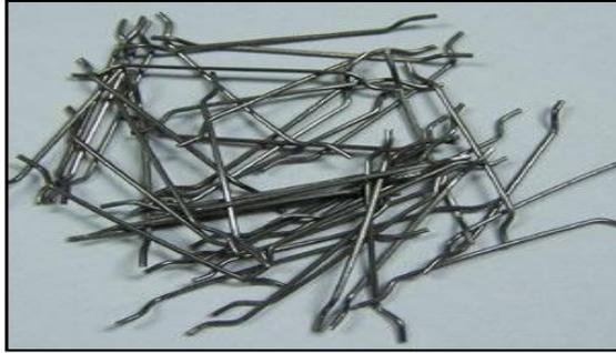
Figure 2: Hooked End Steel Fibre (source by author)
