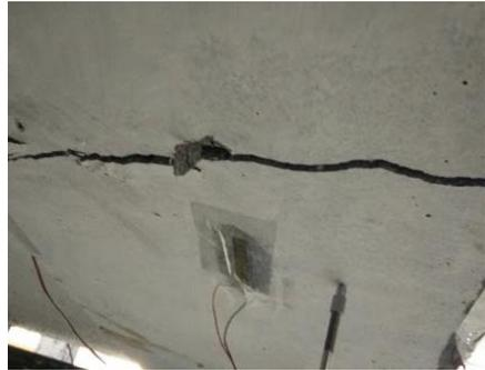
**Figure 9: Crack Pattern of Failed Two-Ribbed Slab (source by author)**
